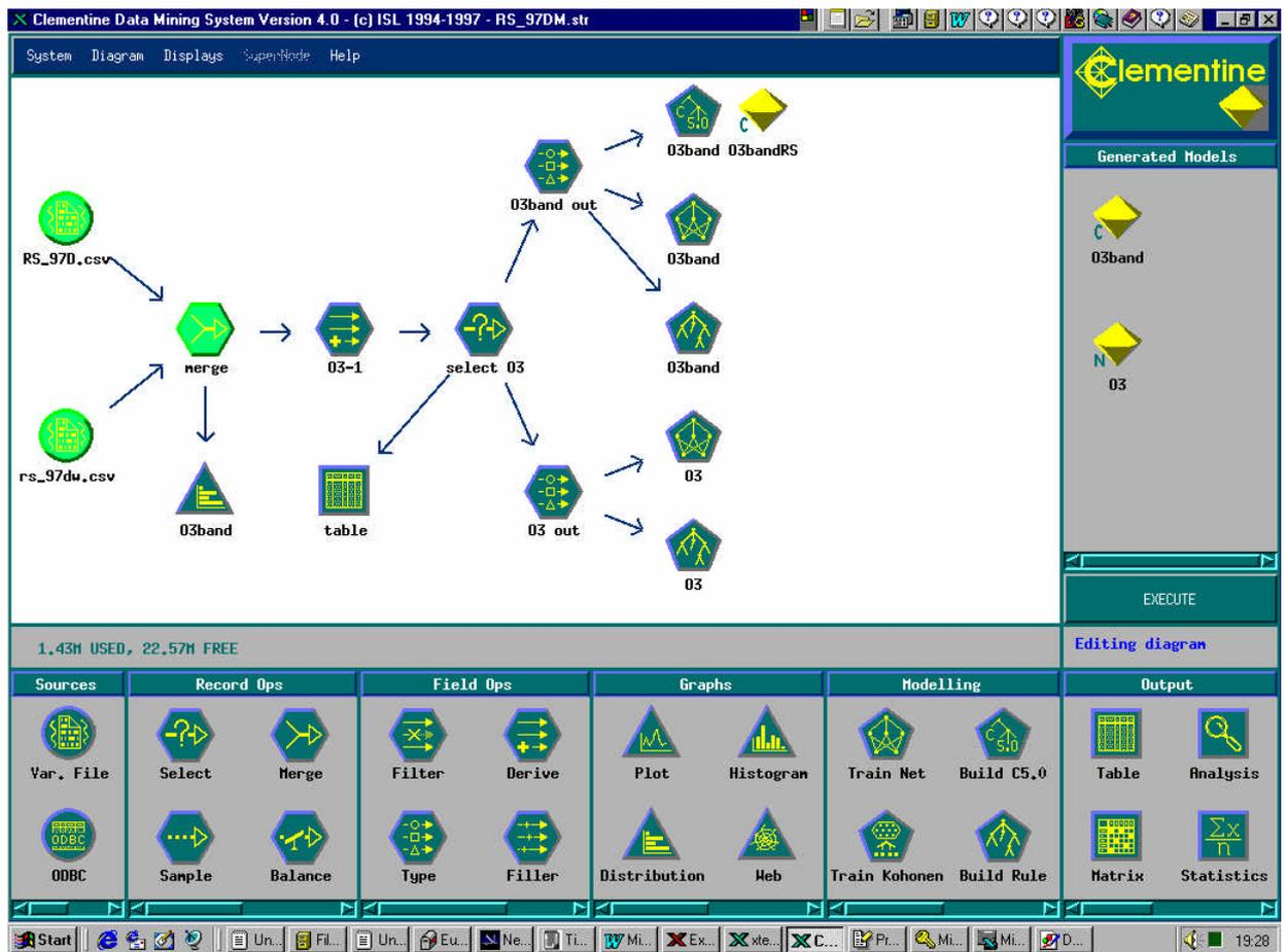
The Clementine user interface: The two source data files of weather and air pollutants measurements are merged, ozone bands selected and models (C5 decision tree and neural net) generated.
