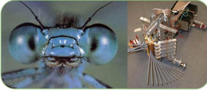
Morphological computation. Facet distribution of insect eye and robot system 'Eyebot' with an artificial compound eye, which can autonomously modify the angular positions of the individual facets. The physical arrangement of the facets — the morphology of the facet eye — performs a kind of 'computation', thus facilitating neural processing.
