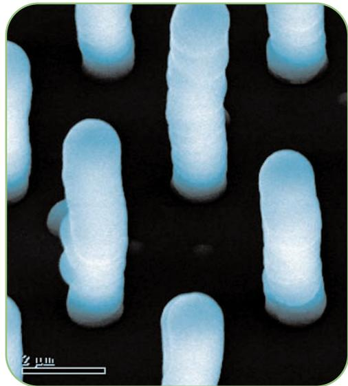
Array of vertically aligned carbon nanotubes grown using plasma enhanced chemical vapor deposition is intercalated with  $\text{SiO}_2$  to provide a bottom-up process for developing interconnects. These vertical interconnects are ideal for DRAM applications and three-dimensional architectures.
