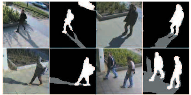
Figure 2: Different parts of the day in sequences at the entrance of Pázmány Péter Catholic University with segmentation results. Above left: in the morning ('am'), right: at noon, below left: in the afternoon ('pm'), right: wet weather.
