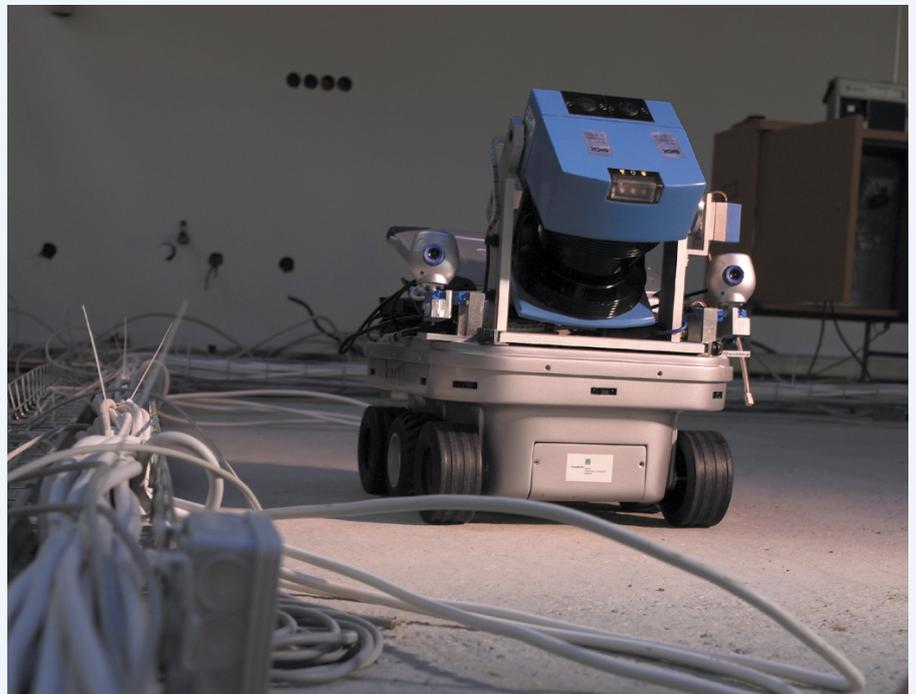
Figure 1: The autonomous mobile robot Kurt3D mapping a construction site.
