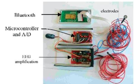
Figure 2: EEG sensor prototype.
