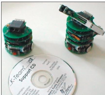
Figure 1: The Khepera robots.
