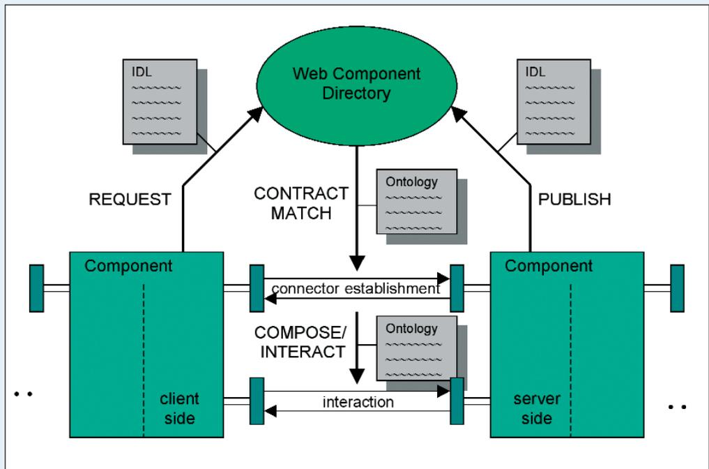
**Web Component Life-Cycle.** A component request might be matched by a server component published in a Web component directory. Successful matching results in direct communication between client and server component to establish a connector for service invocation and reply.
