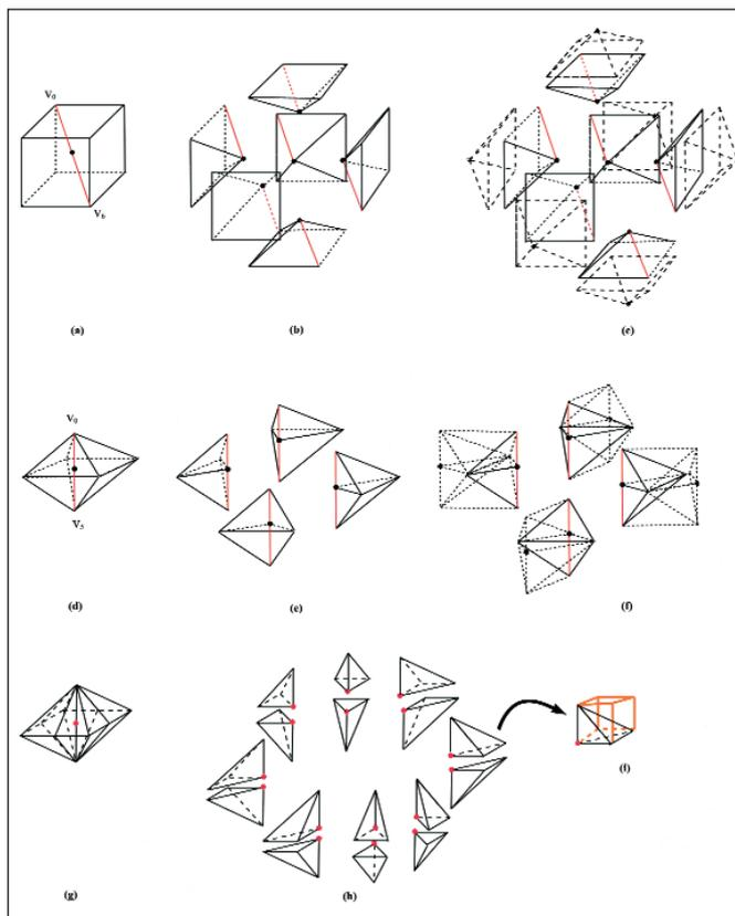
Figure 3: First, second and third level diamonds and respective subdivision and fusion with adjacent cells.
