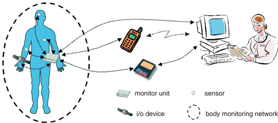
Figure 1: Overview of the Body Monitoring System.
