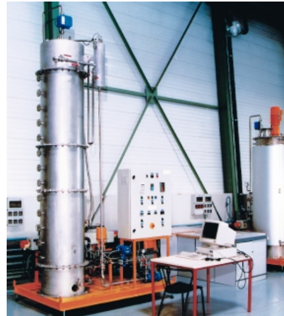
Prototype of an anaerobic digester. Photo: INRA-COMORE.
