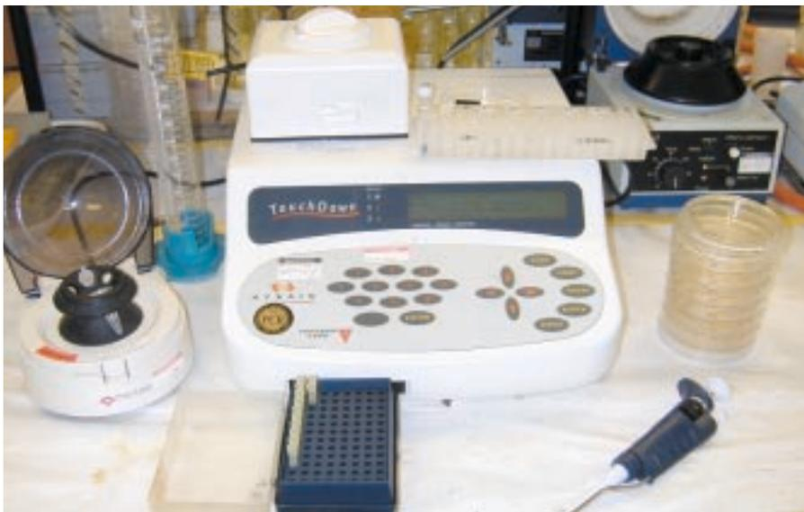
PCR equipment, used to amplify DNA samples.
