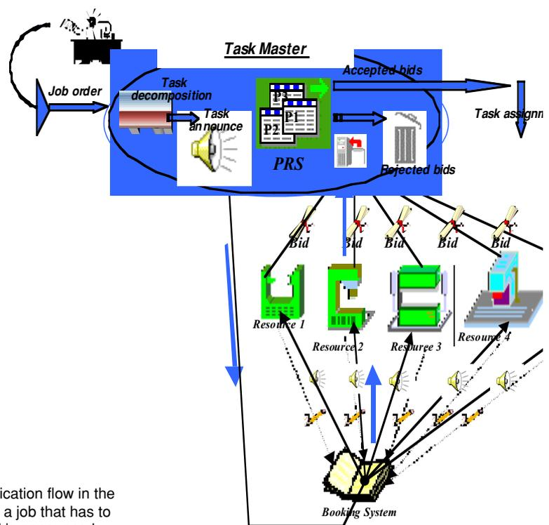
The communication flow in the system when a job that has to be performed is announced.
