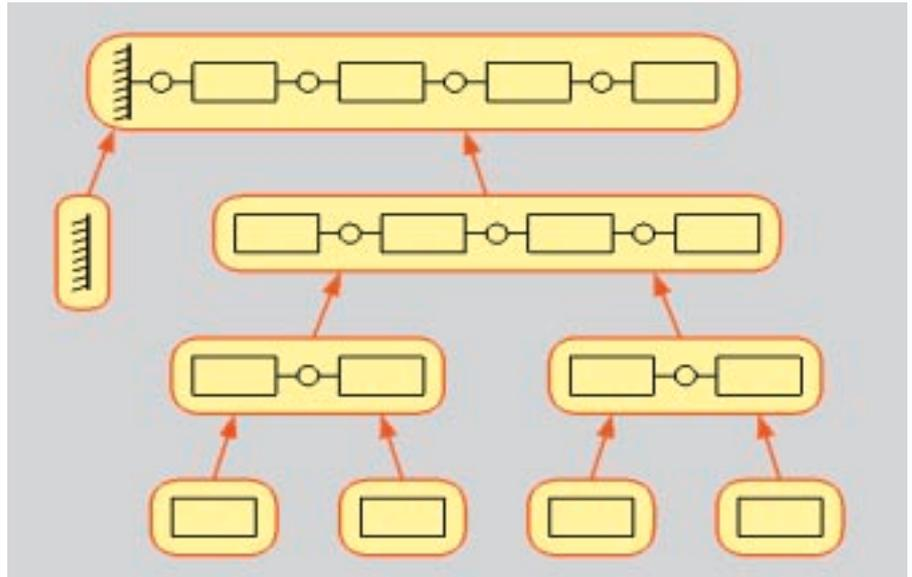
The construction of a rigid-body system from its component bodies by recursive pairwise assembly. The new divide-and-conquer algorithm constructs the equations of motion in the same manner.
