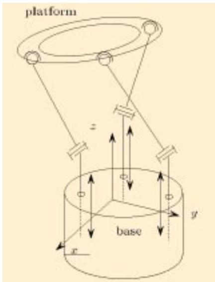
Figure 2: The mechanical architecture of the micro-robot.
