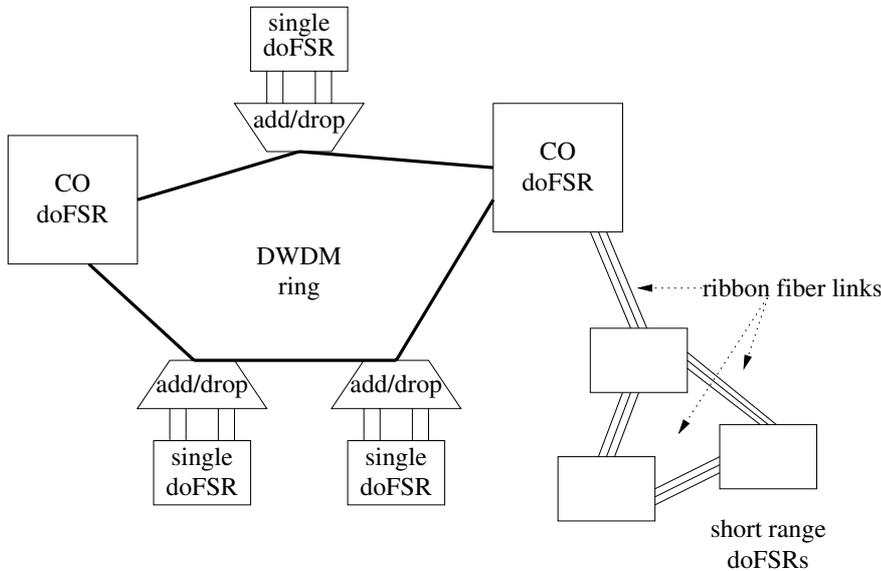
Figure 1: An example of heterogeneous doFSR network architecture.
