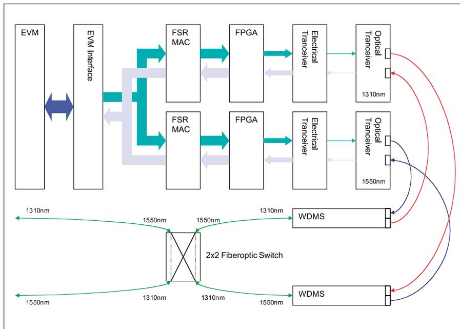
Figure 2: The structure of the prototype system.
