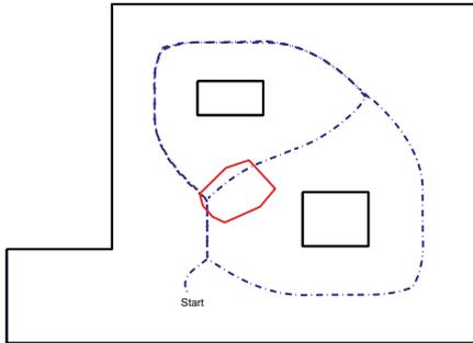
Figure 2: Map building using the Voronoi Diagram.
