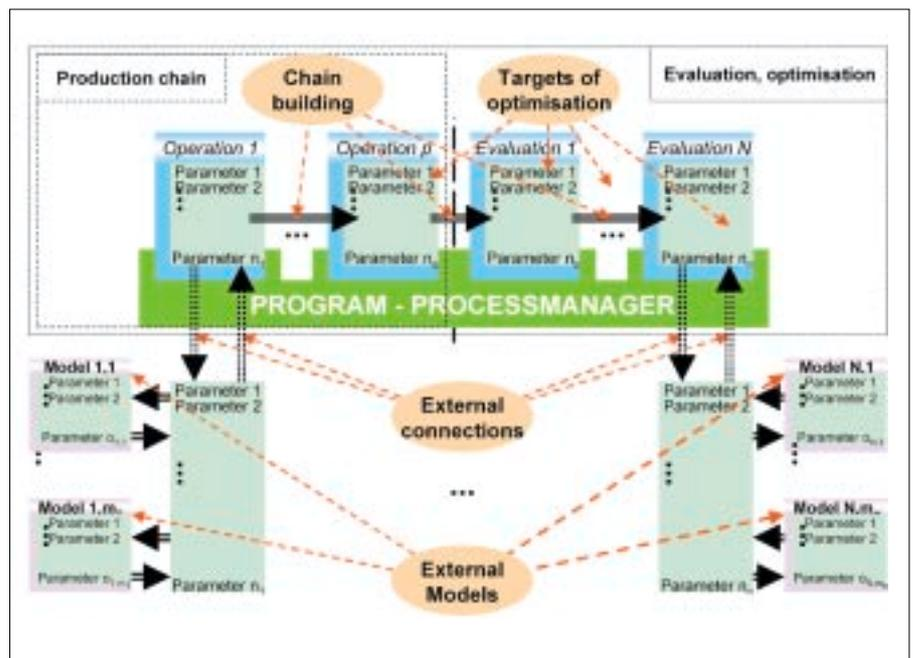
Figure 2: Hybrid modelling and optimisation of process chains by ProcessManager
