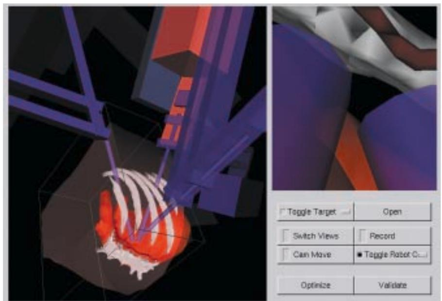
The software designed in the Chir team for the planning and simulation of surgical interventions. Upper right: the endoscopic view, left: the external positioning the robot in the thoracic cage.
