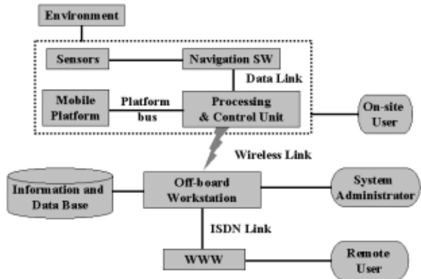
Figure 2: TOURBOT system architecture.
