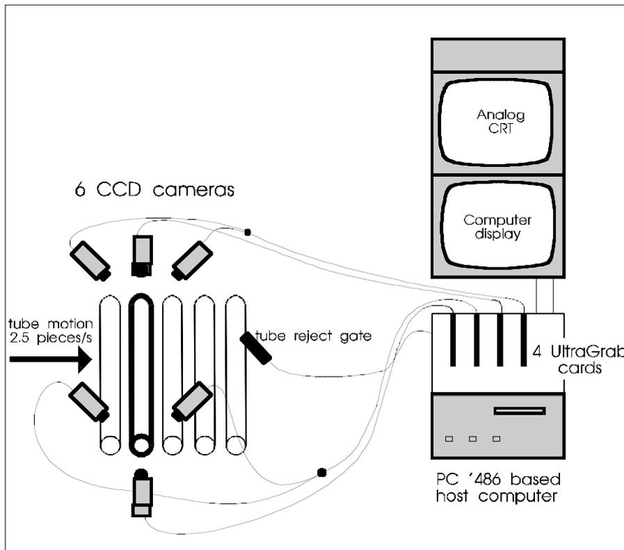
Figure 2: The vision system for testing light tubes.
