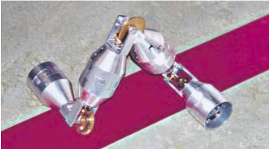
The joints are designed to have special kinematic properties simplifying control, and allowing efficient locomotion. For instance, using the configuration illustrated in the picture, the snake robot can move on flat surfaces without slip friction.
