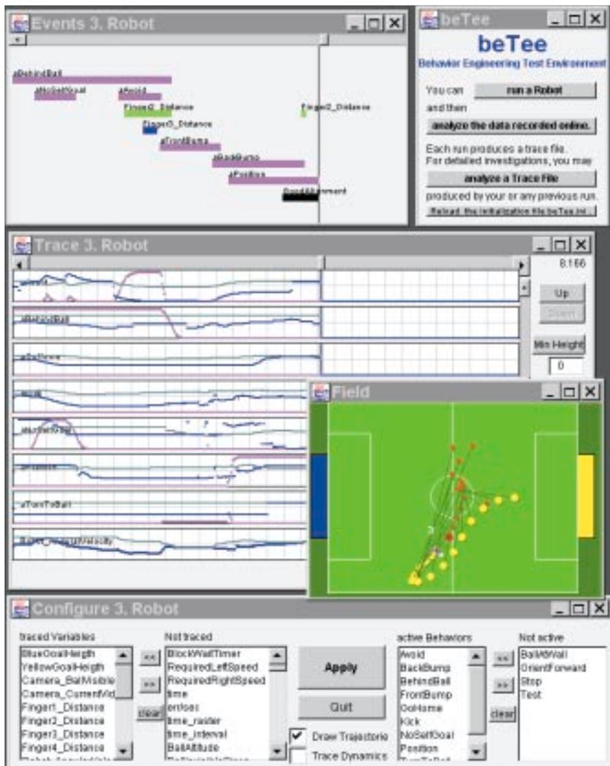
Figure 3: Real-time monitoring tool beTee with symbolized playground, variable state waveforms and event traces.
