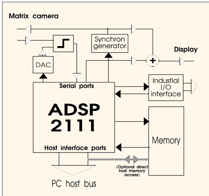
Figure 1: The layout of the UltraGrab card.
