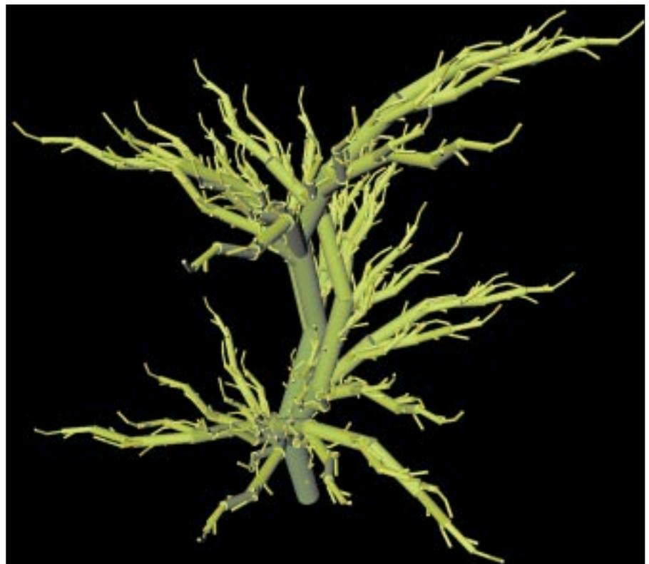
A rigid-body system with 1024 bodies and fractal tree connectivity, used to test the correctness and accuracy of dynamics calculation algorithms.
