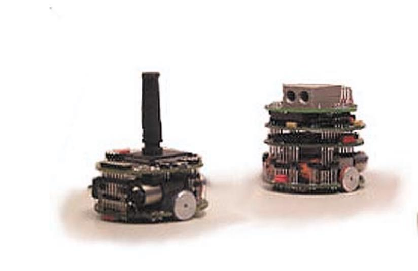
The predator and prey robots consist of two Khepera robots. The predator is equipped with a vision module while the prey has a maximum available speed set to twice that of the predator. Both species were also provided with eight infrared proximity sensors (six on the front side and two on the back). Khepera has been developed at the Laboratory of Microcomputing of the Swiss Federal Institute of Technology (EPFL) in Lausanne.
