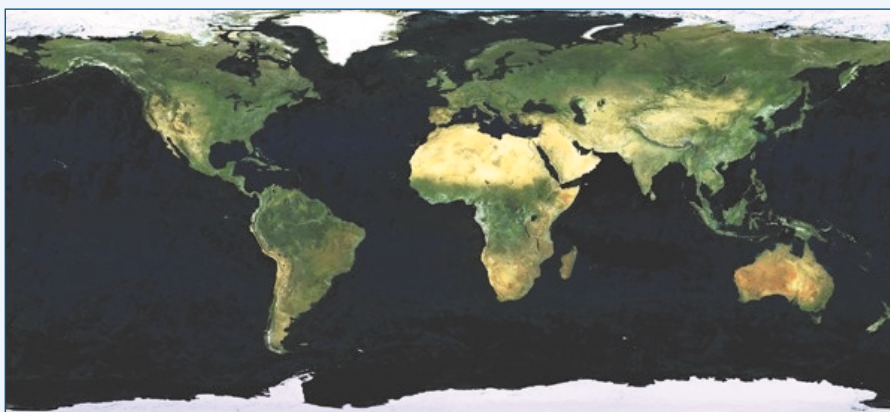
Figure 1: MERIS mosaic image using data from the months of May, July, October and November 2004. This image is made up of true colour images using four out of 15 MERIS spectral bands taken from Envisat (bands 2,3,5 and 7) with data combined from the selected separate orbital segments with the intention of minimizing cloud cover as much as possible by using the corresponding data flags. In total, more than 1 TeraByte of data was processed to generate a final image of about 1 GigaByte.
