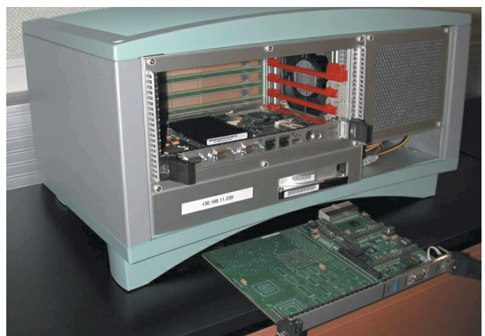
Figure 3: An OAN prototype node is fitted into a standard CompactPCI-frame.
