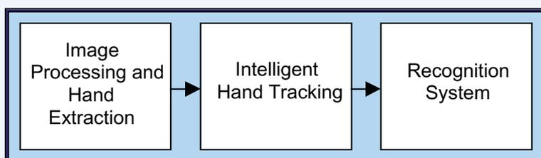
Figure 1: A bimanual movement recognition system.
