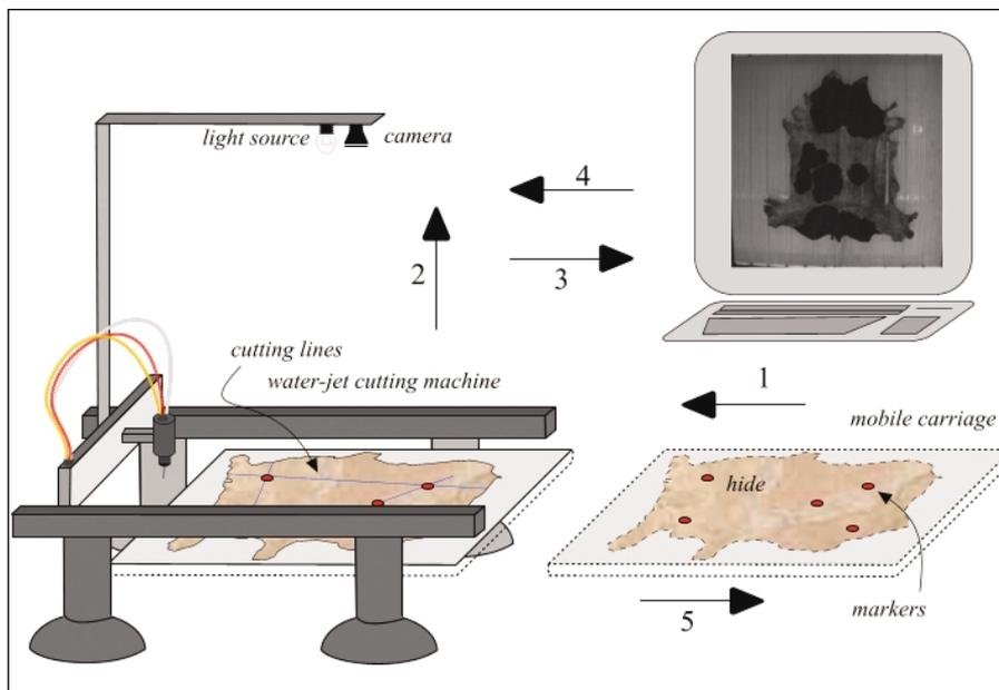
Figure 1: The Cutting System.
