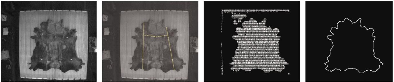
Figure 2: a) The input image; b) Cutting lines; c) detection of inside points; d) contour.
