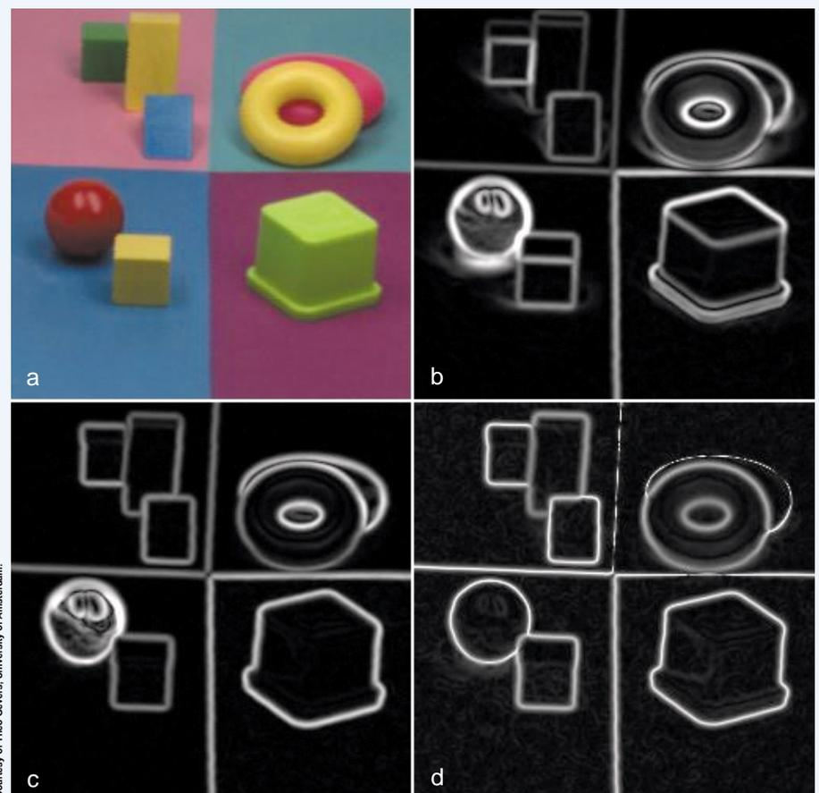
Figure 1: Invariants for color separating shadow (b), highlights (c), and true object contours (d) from all contours (a).
