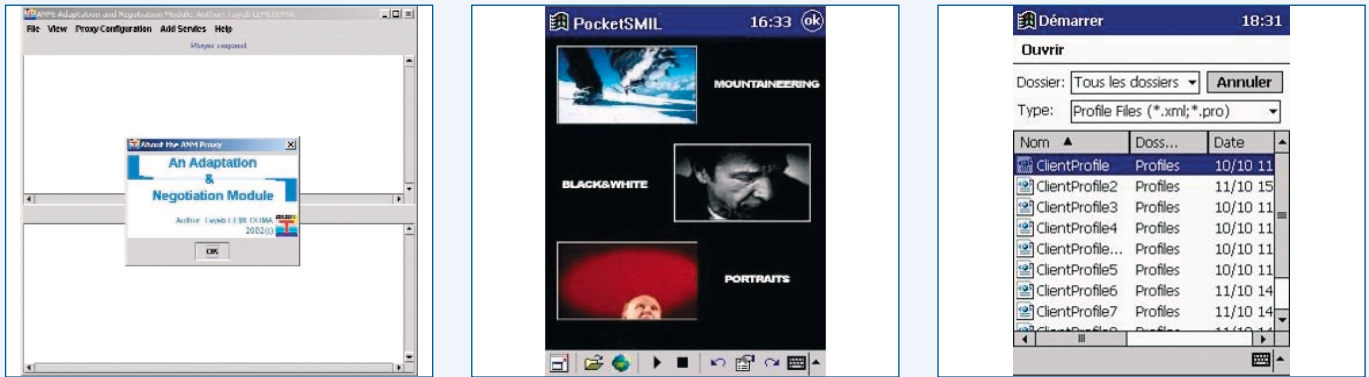
Figure 2: NAC entities: the ANM proxy, Pocket SMIL and the UCM module. From left to right: the proxy; Pocket SMIL, an embedded multimedia player (centre); the User Context Module (right).
