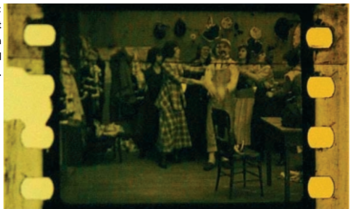
Figure 1: A typical worn-out film-frame with damaged perforation.
