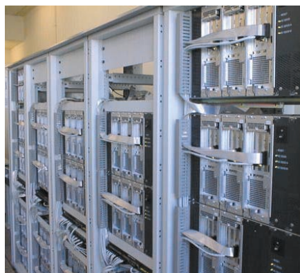
A snapshot of the cluster at the Vrije Universiteit, clearly showing the Myrinet cables (courtesy Henri Bal, Vrije Universiteit, Amsterdam).
