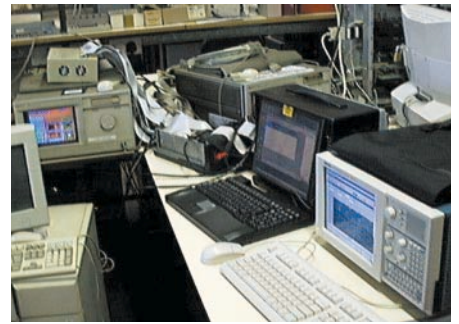
Figure 2: left: tracer/analyzer for the Scalable Coherent Interconnect (see http://www.cs.tcd.ie/coghlan/scieuro/ ), and right: in a heavily instrumented environment.
