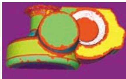
Figure 2: Benchmark part - point cloud segmented.
