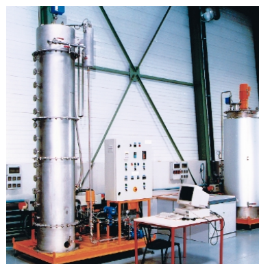
Left: Prototype of an anaerobic digester. Photo: INRA-COMORE. Right: Anaerobic digester at industrial scale.
